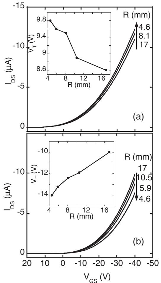
Fig. 3. Transfer curves under (a) compressive and (b) tensile strains with decreasing bending radius from 17 to  $4.6$  mm.  $V_{GS}$  was swept from 20 to  $-40$  V with an application of  $V_{DS} = -40$  V. Insets show the threshold voltage ( $V_T$ ) with changing bending radius.
