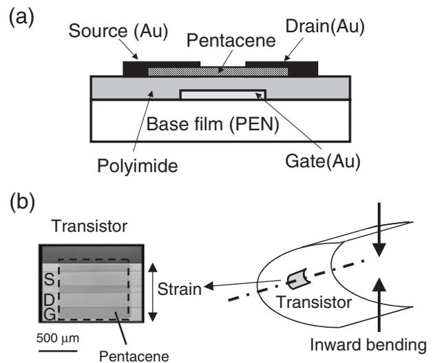
Fig. 1. (a) Cross-sectional illustration of organic FET and capacitor on same PEN base film. (b) Pictures of capacitor and organic FETs with geometry of current applied parallel to the direction of strain.
