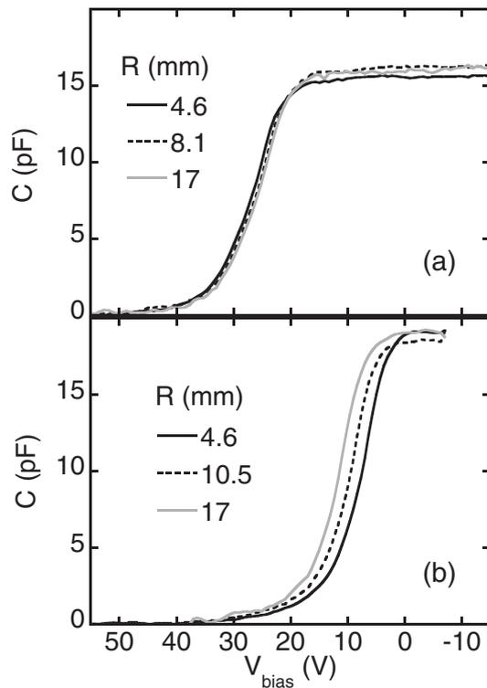
Fig. 4. Capacitance–voltage characteristics of pentacene channel layer with systematically changing bending radius on (a) compression and (b) tension. The measurement frequency was 50 Hz with an AC voltage of 80 mV. The bias DC voltage from the gate electrode was swept from 55 to  $-15$  V at which the source electrode was short-circuited to the drain electrode as a ground.
