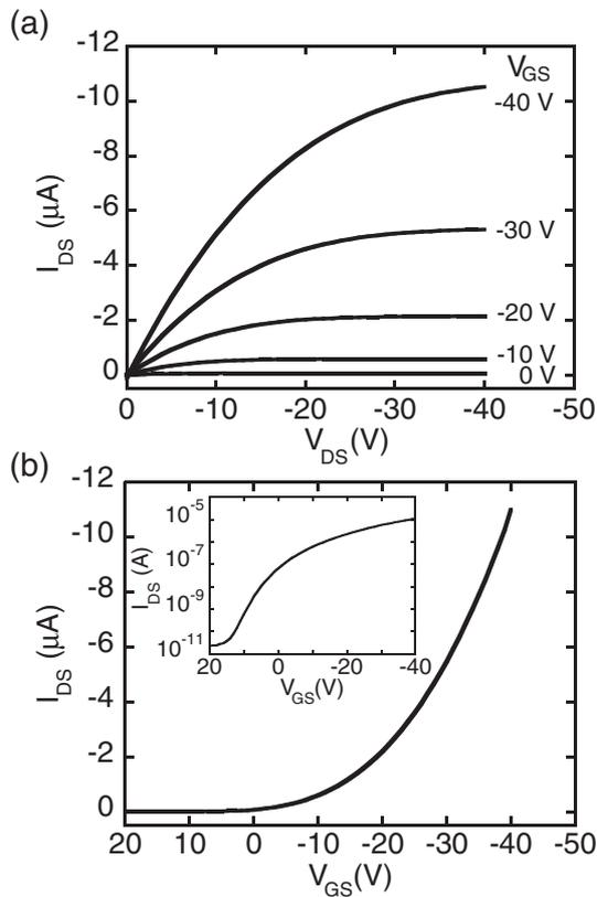
Fig. 2. (a) Typical DC characteristics without stress, which is source-drain current ( $I_{DS}$ ) as a function of source-drain voltage ( $V_{DS}$ ). The gate voltage ( $V_{GS}$ ) was changed from 0 to  $-40$  V in  $-10$  V steps. (b) Corresponding transfer curve with an application of  $V_{DS} = -40$  V. The inset of (b) shows  $I_{DS}$  plotted on a logarithmic scale.
