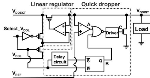
Figure 6. Linear regulator with quick dropper.
