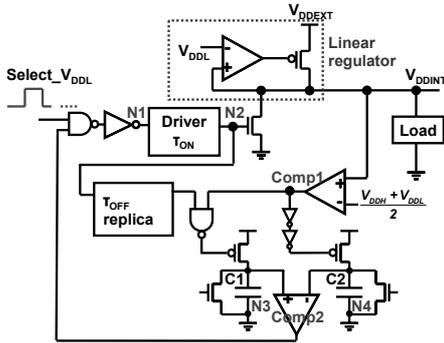
Figure 14. Basic concept of  $V_{DD}$ -hopping accelerator with self-aligned timing generator based on a mirror delay circuit.
