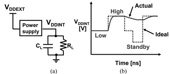
Figure 2. (a) Power supply and equivalent load diagram. (b) Desirable waveform (dotted line) and actual waveform (solid line) for  $V_{DDINT}$ .
