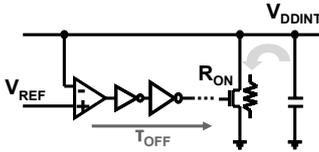
Figure 4. Basic circuit of quick dropper.
