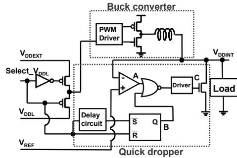
Figure 7. Buck converter with quick dropper.
