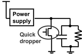
Figure 3. Basic concept of  $V_{DD}$ -hopping accelerator.
