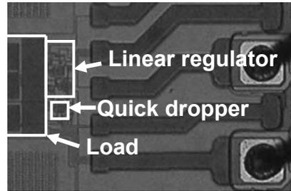
Figure 11. Chip microphotograph of the fabricated linear regulator with the quick dropper. The size of the proposed accelerator is 35x35 $\mu\text{m}$  and it is seen that the accelerator is much smaller compared with a bonding pad.
