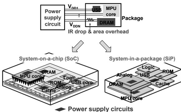
Figure 1. Concept of distributed power supply system.
