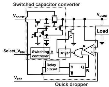
Figure 8. Switched capacitor converter with quick dropper.
