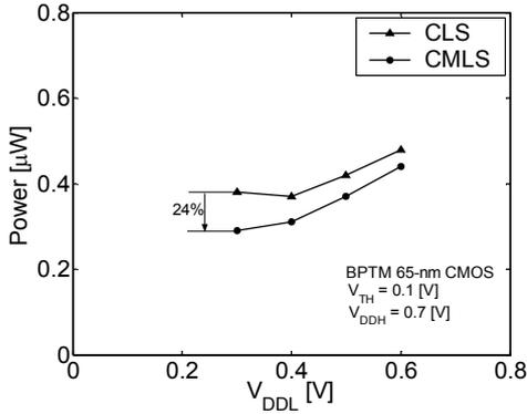
Figure 5 Simulated power consumption of the conventional level shifter and CMLS when  $V_{DDL}$  is varied and  $V_{DDH}$  is fixed. The CLS stands for conventional level shifter. The BPTM 65-nm CMOS model is used. The area overhead of the CMLS is estimated at a value of 4%.
