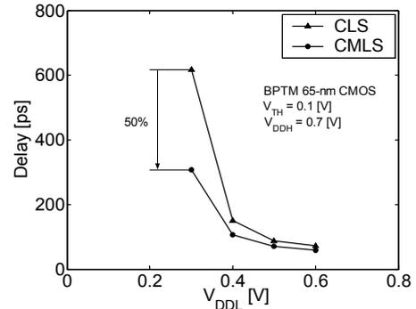
Figure 4 Simulated delay of the conventional level shifter and the CMLS when  $V_{DDL}$  is varied and  $V_{DDH}$  is fixed. The CLS stands for conventional level shifter. The BPTM 65-nm CMOS model is used.
