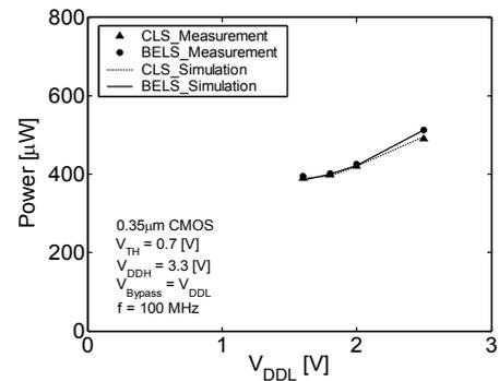
Figure 8 Power of the conventional and proposed level shifter when output voltage  $V_{DD} = V_{DDH}$ . The CLS stands for conventional level shifter.
