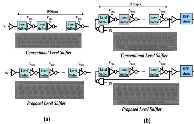
Figure 10 (a) Schematics and microphotographs of level shifter chains for power measurement. (b) Schematics and microphotographs of level shifter ring oscillators for delay measurement.
