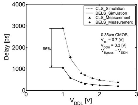
Figure 7 Delay of the conventional and proposed level shifter when the output voltage  $V_{DD}=V_{DDL}$ . The CLS stands for the conventional level shifter.
