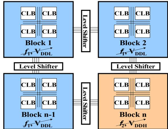
Figure 1 Block-level  $V_{DD}$ -hopping
