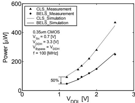
Figure 9 Power of the conventional and proposed level shifter when output voltage  $V_{DD}=V_{DDL}$ . CLS stands for conventional level shifter.
