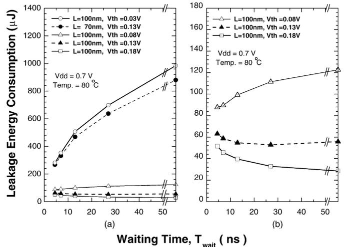
Fig. 10. (a) Simulated average leakage energy consumption of 64-bit CLA as a function of waiting time before entering sleep mode for application B with five different device conditions. (b) The three different threshold voltage conditions with  $L = 100$  nm are redrawn with more detail energy scale.
