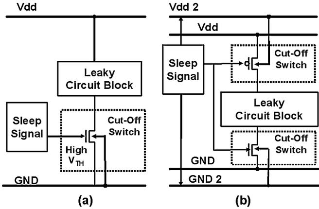
Fig. 1. Block diagrams of two cut-off schemes. (a) MTCMOS. (b) VTCMOS.
