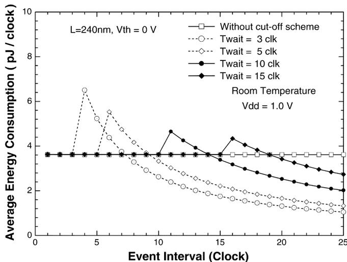
Fig. 12. Measured average energy consumption as a function of event interval with respect to various waiting times.
