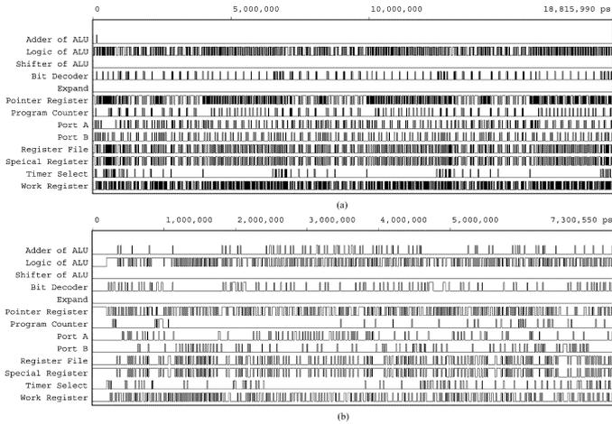
Fig. 4. Block activation signals for two different applications of the 8-bit RISC microprocessor. (a) Application A: LCD driver. (b) Application B: Toy controller.
