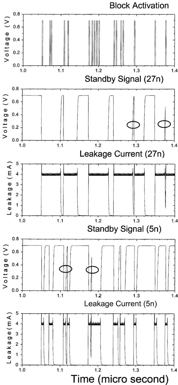
Fig. 9. Simulated leakage current behaviors of 64-bit CLA for application B with the self-timed cut-off controller shown in Fig. 8. Time conditions marked by a circle means energy-consuming events by the self-cut-off scheme. The others are energy-saving events.
