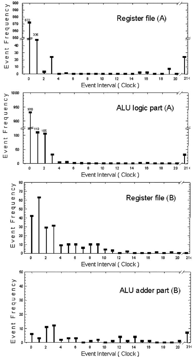
Fig. 5. Extracted event frequency as a function of event interval (the number of clocks between two adjacent block activations). A and B represent two applications, as shown in Fig. 4.
