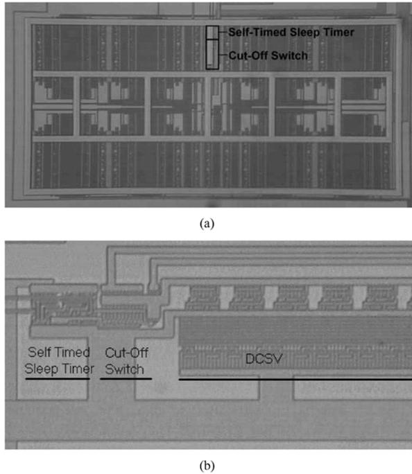
Fig. 11. Microphotographs of (a) fabricated test chip of 64-bit carry-look-ahead adder with self-timed cut-off switch, and (b) differential cascode voltage switch (DCSV) logic.
