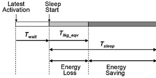
Fig. 6. Definition of notations to calculate a criterion of statistical energy saving.
