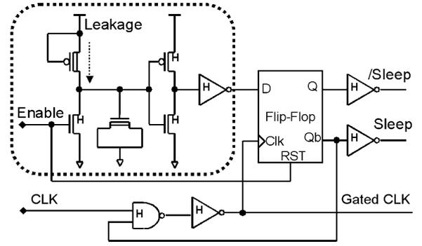
Fig. 8. Self-timed cut-off controller used in the simulations and experiments. Transistors marked H represent high threshold voltage transistors.
