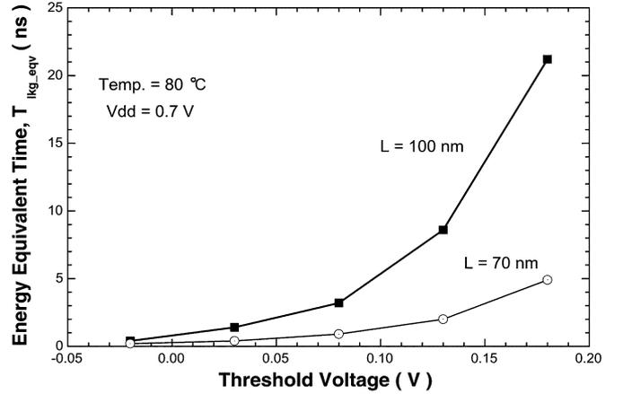
Fig. 3. Estimated leakage energy equivalent times with the variations of threshold voltage and channel length.
