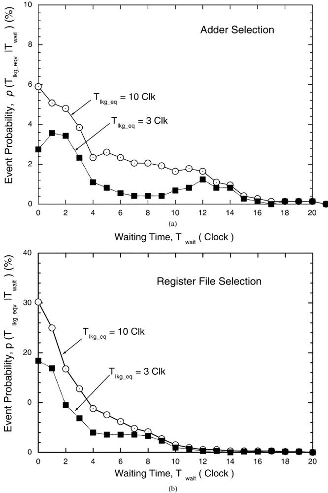
Fig. 7. Conditional probability of activation as a function of waiting time. Adder and register file of application B. (a) Adder. (b) Register file.
