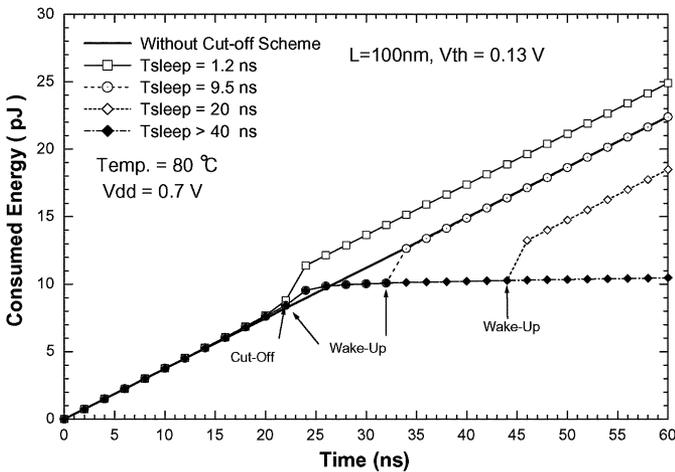
Fig. 2. Simulated results of the 64-bit carry-look-ahead adder with respect to various sleep times. It is derived from the viewpoint of  $V_{DD}$ , so the discharge current to ground is added next recharge current.
