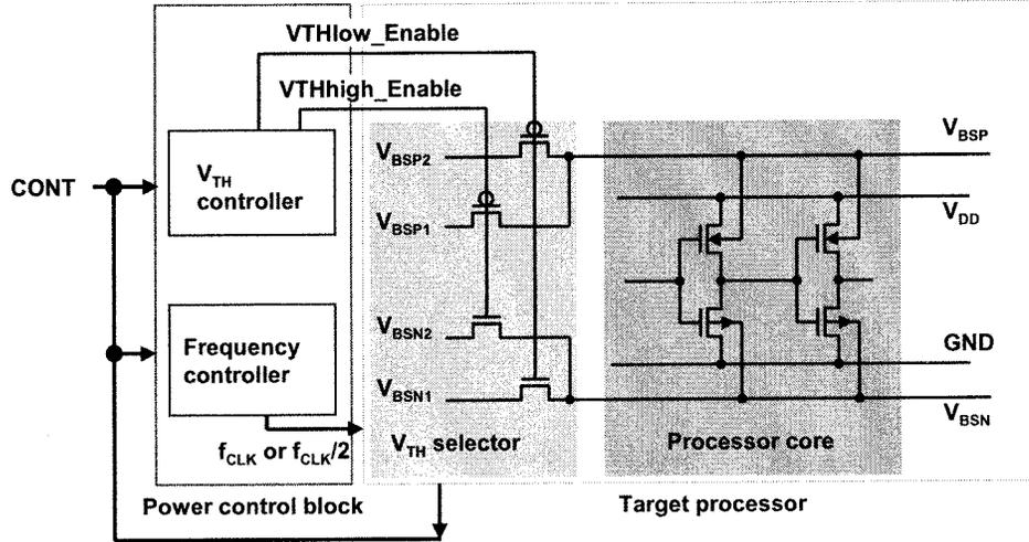
Fig. 4. Schematic diagram of  $V_{TH}$ -hopping.
