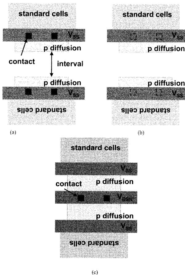
Fig. 12. Place and route using conventional standard cells.
