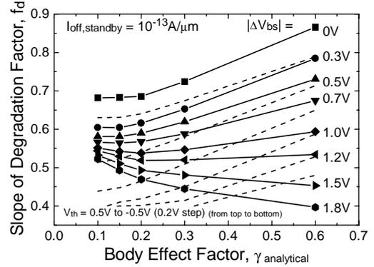
**Fig. 10** The dependence of the slope of the degradation factor on the body effect factor. Contour lines of the threshold voltage are also shown.
