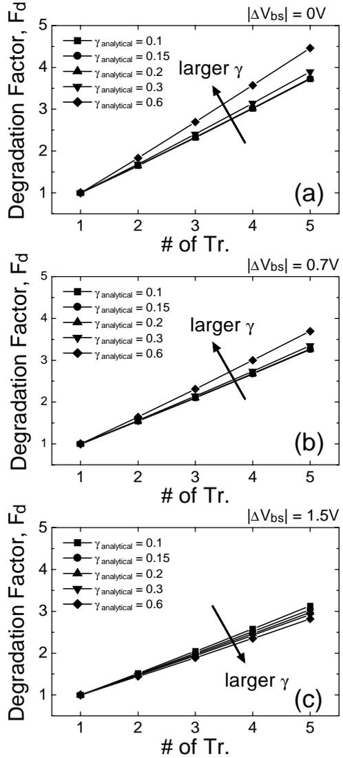
Fig. 6 The dependence of the degradation factor on the number of the series connected MOSFETs. (a)  $|\Delta V_{bs}| = 0V$  (normal MOSFET), (b)  $|\Delta V_{bs}| = 0.7V$  and (c)  $|\Delta V_{bs}| = 1.5V$ .
