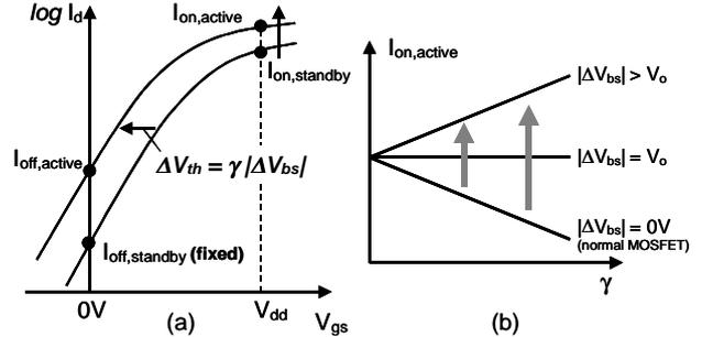
**Fig. 1** (a) Schematics of VTCMOS characteristics. Utilizing the body effect, *on*-current in the active mode ( $I_{on,active}$ ) can be enhanced, while *off*-current in the stand-by mode ( $I_{off,standby}$ ) is fixed. (b)  $\gamma$  dependence of  $I_{on,active}$  with the fixed  $I_{off,standby}$ . When  $|\Delta V_{bs}|$  is larger  $V_o$ , larger  $\gamma$  results in higher *on*-current.
