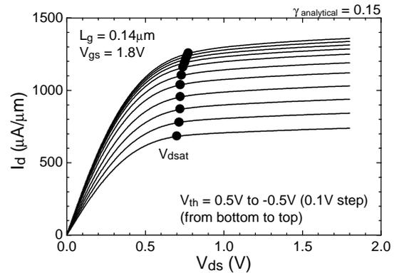
**Fig. 11**  $I_d$ - $V_{ds}$  characteristics of devices with various  $V_{th}$ 's and the same  $\gamma$  value ( $\gamma = 0.15$ ).  $V_{dsat}$  in each device is shown by a dot.
