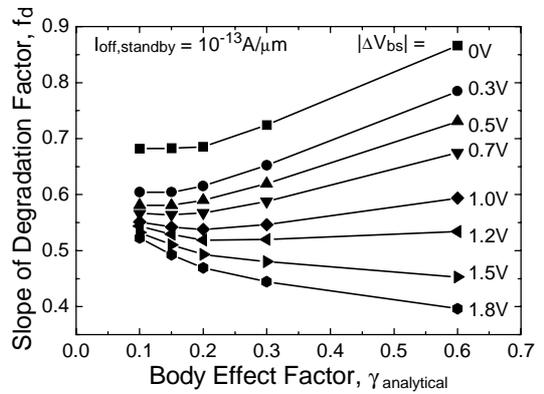
Fig. 7 The dependence of the slope of the degradation factor ( $f_a$ ) on the body effect factor.
