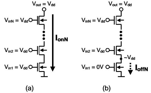
**Fig. 3** Schematics of the series connected circuits and the definitions of (a) *on*-current and (b) *off*-current.
