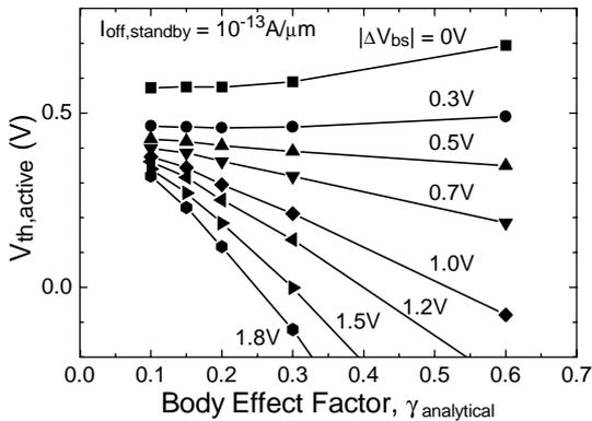
**Fig. 9** The dependence of the threshold voltage in the active mode ( $V_{th,active}$ ) on the body effect factor. When  $|\Delta V_{bs}|$  is large, larger  $\gamma$  results in lower  $V_{th,active}$ .
