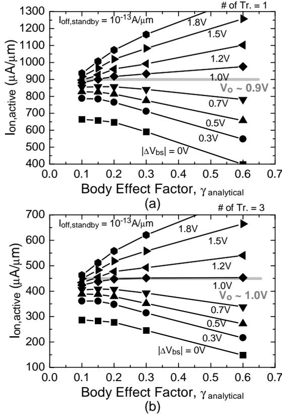
**Fig. 4** The dependence of the active *on*-currents on the body effect factor in VTCMOS. (a) Single device ( $N = 1$ ) and (b) series connected circuit ( $N = 3$ ). In each case, the threshold voltage is adjusted so that the stand-by *off*-current is fixed to  $10^{-13} A/\mu m$  with given  $|\Delta V_{bs}|$ .
