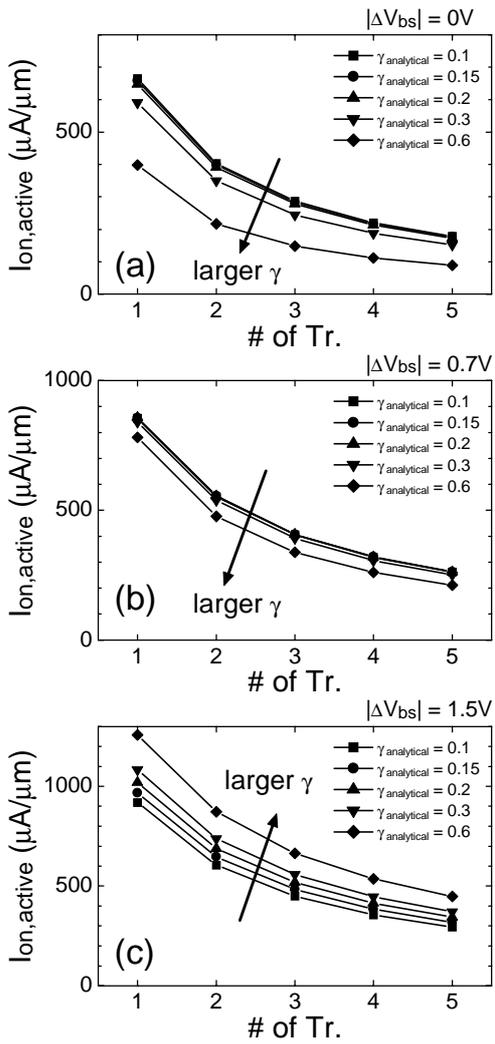
Fig. 5 The dependence of the active *on*-current on the number of the series connected MOSFETs. (a)  $|\Delta V_{bs}| = 0V$  (normal MOSFET), (b)  $|\Delta V_{bs}| = 0.7V$  and (c)  $|\Delta V_{bs}| = 1.5V$ .
