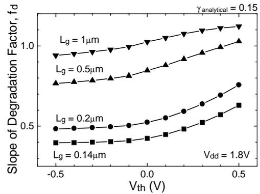
**Fig. 15** The dependence of the slope of the degradation factor on  $V_{th}$  for devices with various gate lengths.
