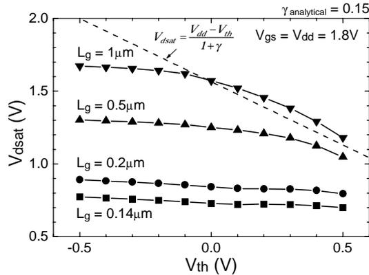
**Fig. 13** The dependence of  $V_{dsat}$  on  $V_{th}$  for devices with various gate lengths. Comparison with an analytical form for the long channel devices is also shown.  $V_{dsat}$  varied linearly with  $V_{th}$  in long channel devices. On the other hand,  $V_{dsat}$  remains almost constant in short channel devices due to velocity saturation.
