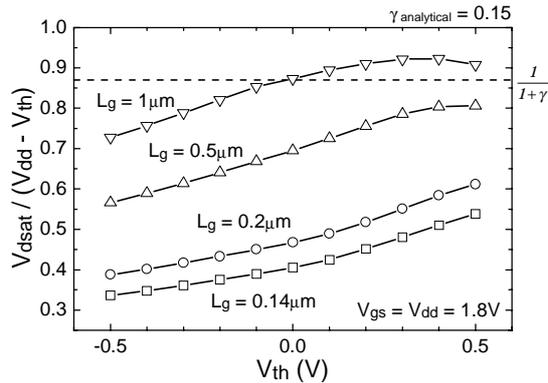
**Fig. 14** The dependence of the ratio of  $V_{dsat}$  to  $V_{dd}-V_{th}$  for devices with various gate lengths. Comparison with an analytical form for the long channel devices is also shown. The ratio rapidly decreases with  $V_{th}$  in short channel devices compared with long channel devices.
