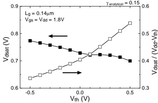
**Fig. 12** The  $V_{th}$  dependence of the saturation voltage ( $V_{dsat}$ ) and ratio of  $V_{dsat}$  to gate drive ( $V_{dd}-V_{th}$ ). As  $V_{th}$  decreases,  $V_{dsat}$  increases only slightly, resulting in reduction of the ratio.
