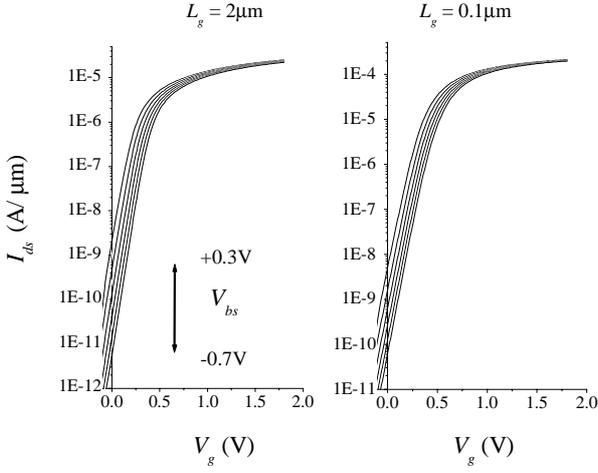
**Figure 2.** Measured  $I_{ds}$  versus  $V_g$  characteristics of  $n$ -type MOSFETs as a function of  $V_{bs}$ .  $10\text{mV}$   $V_{ds}$  was applied for the measurements.
