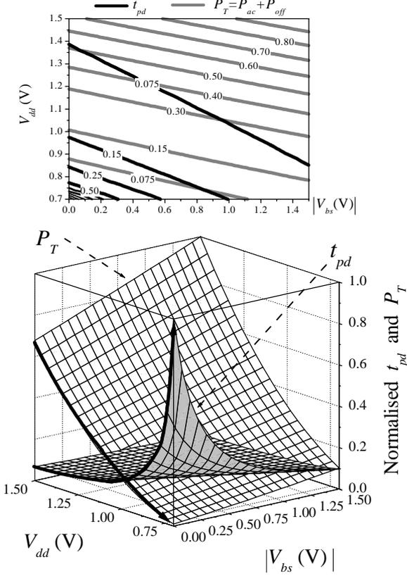
**Figure 4.** Normalized gate delay time ( $t_{pd}$ ) and total power ( $P_T$ ) as a function of  $V_{bs}$  and  $V_{dd}$  at a constant  $I_{off}(s)$  of  $10^{-13}$  A/ $\mu\text{m}$ . In these calculations,  $S = 80\text{mV/decade}$ ,  $\gamma = 0.2$  and  $\alpha = 1.3$  are used. The upper plot shows the contour lines of  $t_{pd}$  and  $P_T$  in the  $V_{bs} - V_{dd}$  plane
