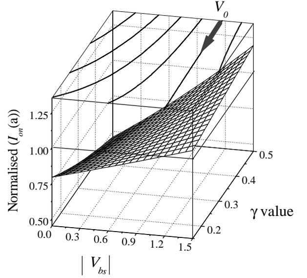
**Figure 5.** Calculated  $I_{on}(a)/I_o$  and its contour map onto the  $\gamma - V_{bs}$  plane. In this calculation, the values of  $\alpha$  and  $V_{dd}$  are 1.5 and 1.5V respectively.  $I_{off}(s)$  is fixed at a  $10^{-13}$  A/ $\mu\text{m}$ .
