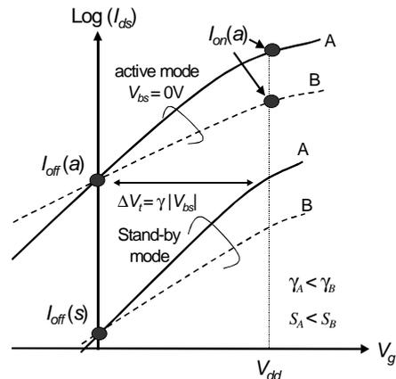
Figure 1. Schematic description of the characteristics of VTCMOSs whose  $\gamma$  and  $S$  are different. For easy comparison and simplicity, off-currents in the stand-by and active modes are set the same. Device A has higher on-current ( $I_{on}(a)$ ) due to its smaller  $S$  but requires larger  $V_{bs}$  than device B to attain the same stand-by off current ( $I_{off}(s)$ ) due to the smaller  $\gamma$ . This is quantitatively understood using (2) and (3) in the text.
