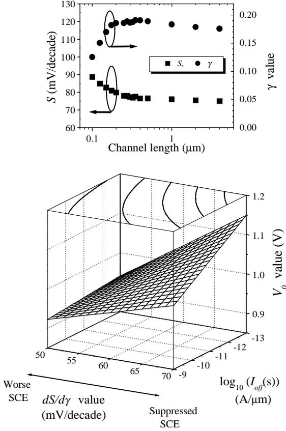
**Figure 6.** Calculation of the characteristic  $|V_{bs}| (=V_0)$ .  $\gamma = 0.3$  and  $V_{dd} = 1.5V$ . The upper plot shows the measurements of  $S$ , and  $\gamma$  values as a function of channel length. Equation (10) is used for  $dS/d\gamma$ .
