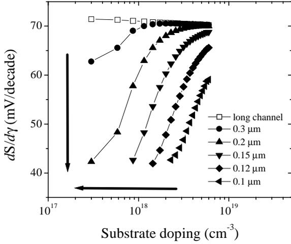
**Figure 7.** Analytical calculation of  $dS/d\gamma$  in an uniformly doped VTCMOS, as a function of channel length and substrate doping concentration. The thick arrows indicate directions where the short channel effect becomes worse.  $|V_{bs}| = 1V$ .  $t_{ox} = 40\text{\AA}$ .
