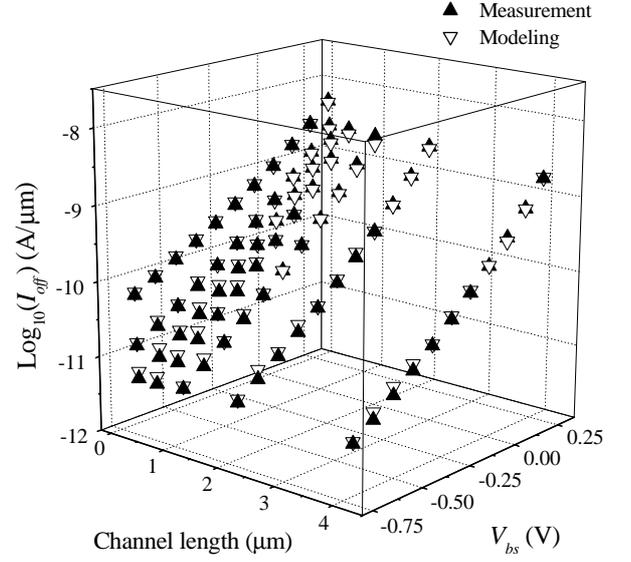
**Figure 3.** Comparison between the measured and modeled  $I_{off}(s)$  data as a function of  $V_{bs}$ . Note that the modeled results are also in excellent agreement in the positive substrate bias ( $+V_{bs}$ ) regime.
