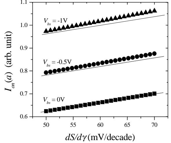
**Figure 8.** Enhancement of  $I_{on}(a)$  at  $\gamma = 0.3$  under three different substrate biases, as a function of  $dS/d\gamma$ . Note that  $I_{off}(s)$  is fixed at  $10^{-13}\text{A}/\mu\text{m}$ . Other modeling parameters are the same with those used for Fig 5. The three lines represent the slope of  $I_{on}(a)$  at  $V_{bs} = 0V$ .
