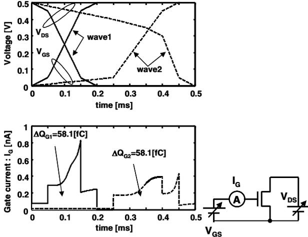
Fig. 3 Method to obtain  $C_{G,eff}$  and  $\Delta Q_G$  dependence on the waveforms of gate voltage and drain voltage
