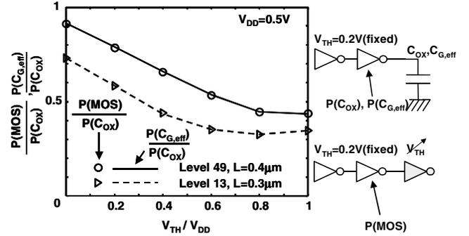
Fig. 4 Comparison of power estimated by using  $C_{G,eff}$  ( $P(C_{G,eff})$ ),  $C_{OX}$  ( $P(C_{OX})$ ) and real MOS gate ( $P(MOS)$ )
