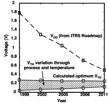
Fig. 8 Future trend of optimum  $V_{DD}$  and  $V_{TH}$ [4]
