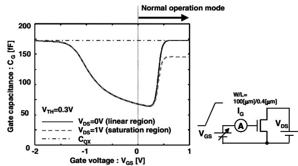
Fig. 1 Dependence of gate capacitance on gate and drain voltage
