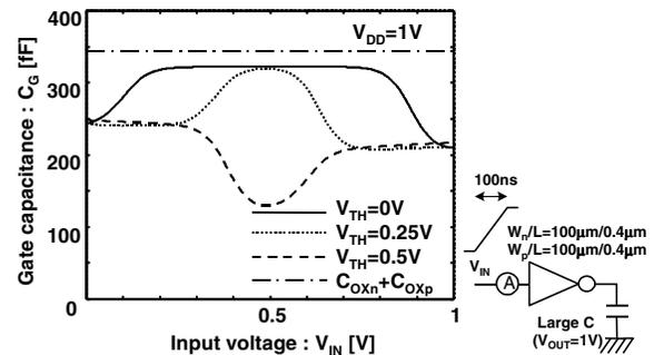
Fig. 2 Dependence of inverter input capacitance on gate voltage and threshold voltage
