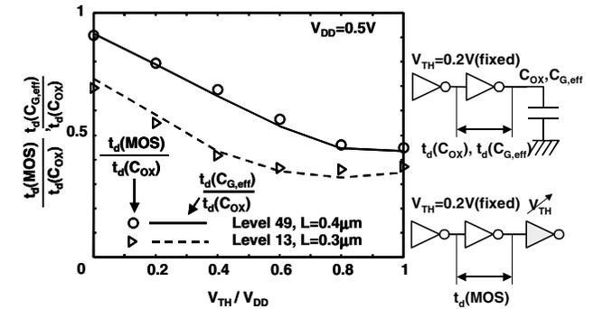
Fig. 5 Comparison of delay estimated by using  $C_{G,eff}$  ( $t_d(C_{G,eff})$ ),  $C_{OX}$  ( $t_d(C_{OX})$ ) and real MOS gate ( $t_d(MOS)$ )
