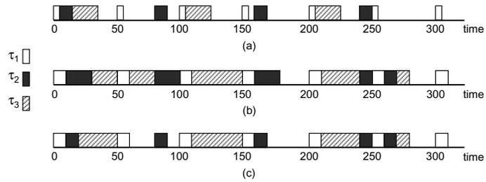
Figure 2. A schedule for the example task set. (a) When tasks always run at their WCETs. (b) When tasks always run at their WCETs on a processor with the speed lowered by half. (c) When the execution times of some task instances are smaller than their WCETs.
