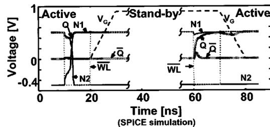
Fig. 7. Operation waveforms of flip-flop with SCCMOS.
