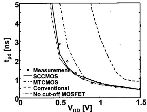
Fig. 8. Measured speed of flip-flops with SCCMOS.
