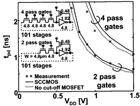
Fig. 11. Measured speed of PTL gates with SCCMOS.
