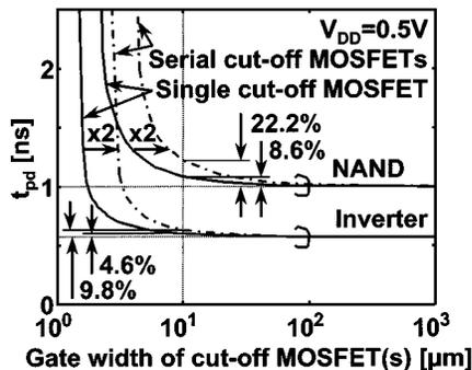
Fig. 5. Simulated speed dependency on gate width of cut-off MOSFET(s) in SCCMOS.
