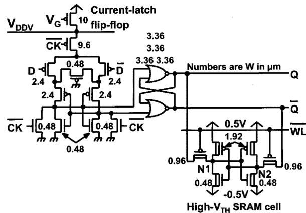
Fig. 6. Flip-flop with SCCMOS.
