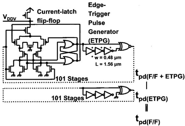
Fig. 9. Method of measuring speed of flip-flops with SCCMOS.
