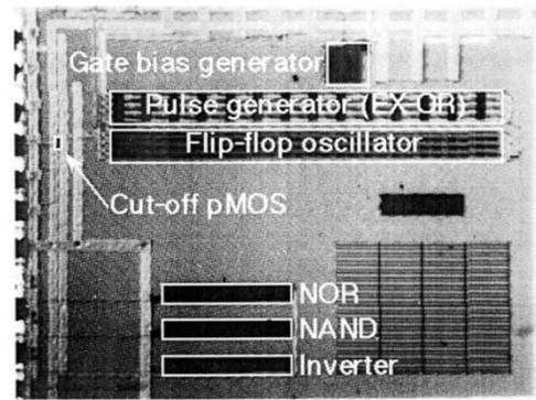
Fig. 3. Microphotograph of fabricated SCCMOS test chip.
