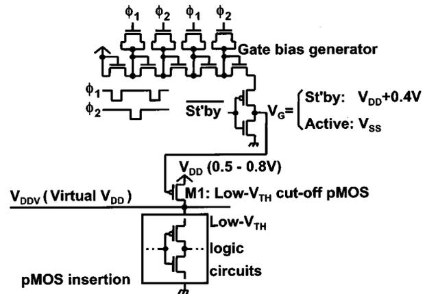
Fig. 1. Concept of SCCMOS.
