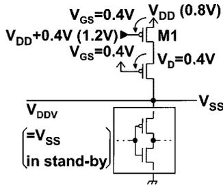
Fig. 2. Gate-oxide reliability problem in SCCMOS.
