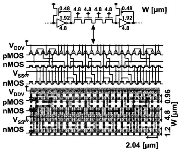
Fig. 10. PTL gate array with SCCMOS.
