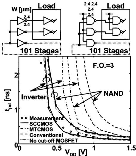
Fig. 4. Measured speed of inverters and 2-NANDs with SCCMOS.
