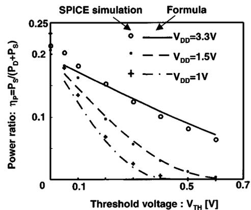
Fig. 13. Power ratio dependence on threshold voltage.
