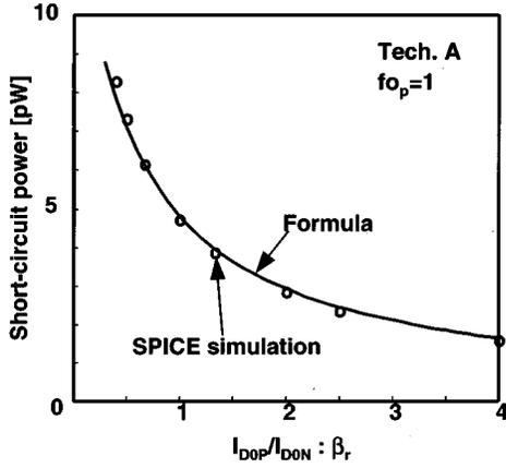
Fig. 5. Short-circuit power dependence on  $\beta_r$ .
