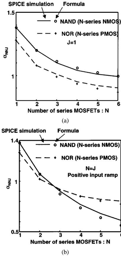
Fig. 10.  $\alpha_{NNJ}$  dependence on number of series MOSFETs (a)  $J = 1$  (b)  $J = N$ .
