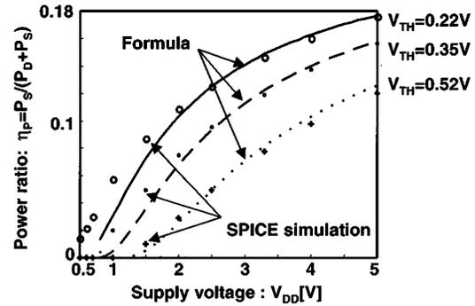
Fig. 12. Power ratio dependence on supply voltage.
