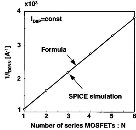
Fig. 9.  $1/I_{D0NN}$  dependence on number of series MOSFETs.
