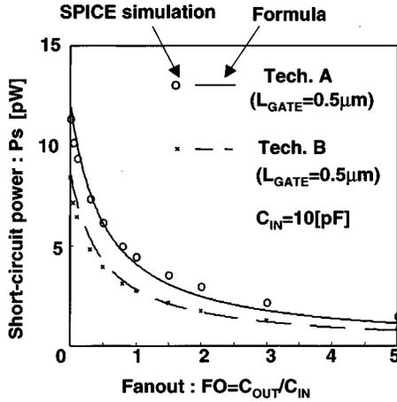
Fig. 2. Short-circuit power dependence on fanout.
