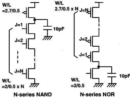
Fig. 7.  $N$  series-connected model structure (SCMS).
