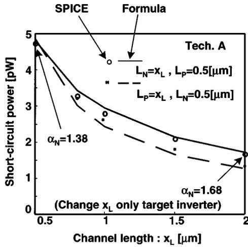
Fig. 6. Short-circuit power dependence on channel length.
