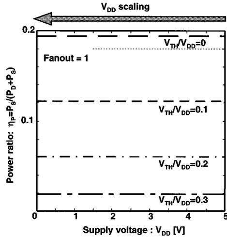
Fig. 15. Power ratio dependence on  $V_{DD}$  scaling.
