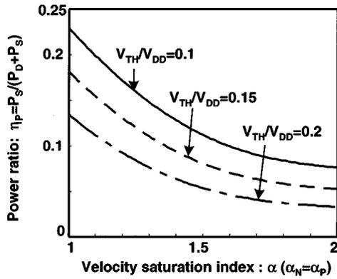
Fig. 14. Power ratio dependence on  $\alpha$ .
