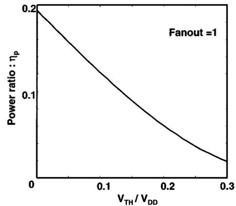
Fig. 16. Power ratio dependence on  $V_{TH}/V_{DD}$ .
