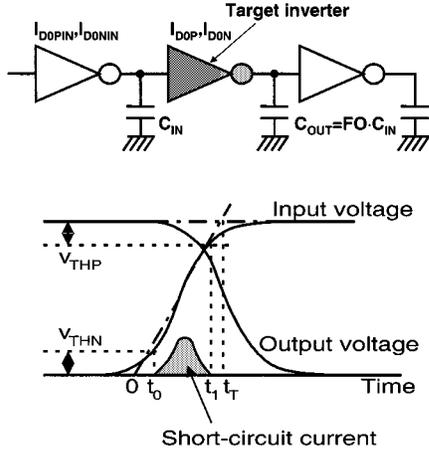
Fig. 1. Voltage waveform of CMOS inverter operation.
