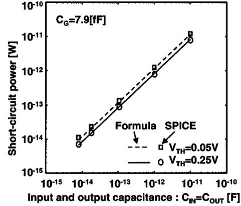
Fig. 3. Short-circuit power dependence on the input and output node capacitance.
