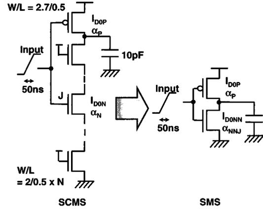
Fig. 8. Approximate  $N$  series-connected MOSFETs (SCMS) with single MOSFET structure (SMS).
