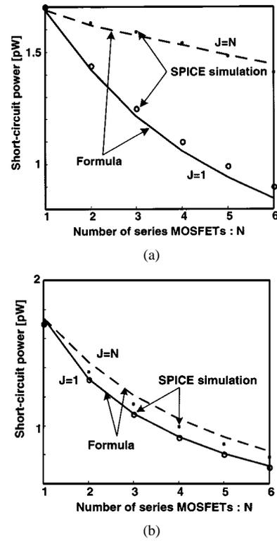
Fig. 11. Short-circuit power dependence on number of series MOSFETs (a)  $N$ -series NAND (b)  $N$ -series NOR.
