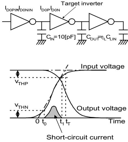
Fig.1 Voltage waveform of CMOS inverter operation
