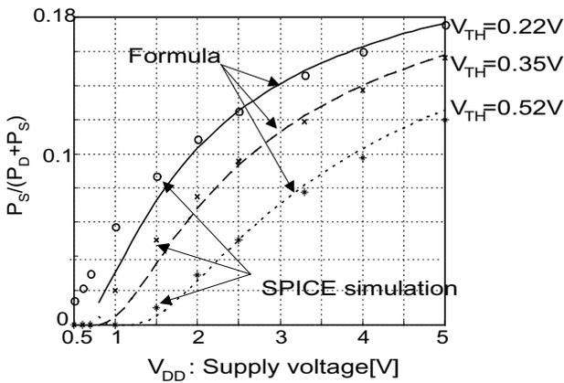
Fig.7 Power ratio dependence on supply voltage
