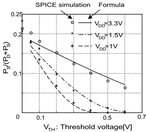
Fig.6 Power ratio dependence on threshold voltage
