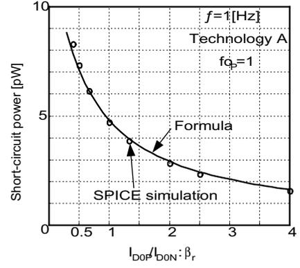
Fig.4 Short-circuit power dependence on  $\beta_r$
