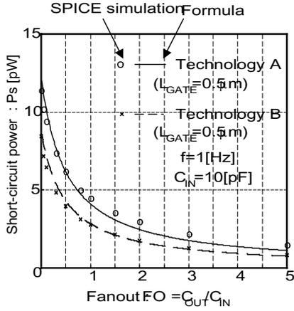
Fig.2 Short-circuit power dependence on fanout( $FO$ )
