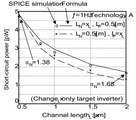
Fig.5 Short-circuit power dependence on channel length
