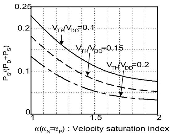
Fig.8 Power ratio dependence on velocity saturation index
