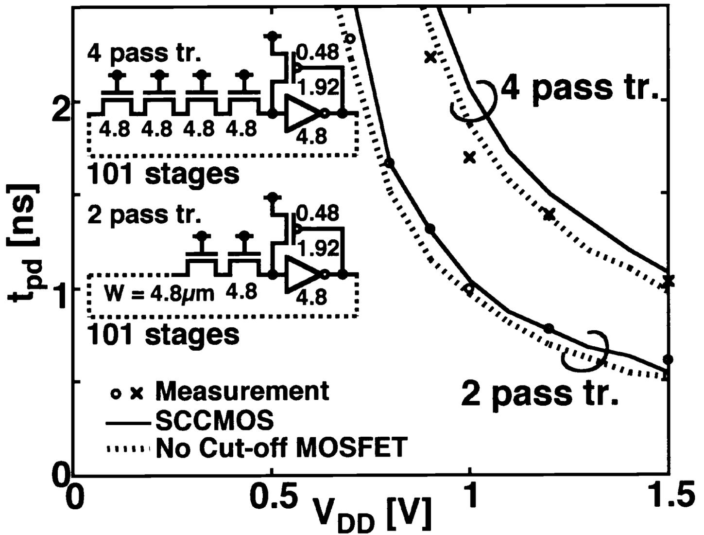
Figure 6: Speed of PTL with SCCMOS.
