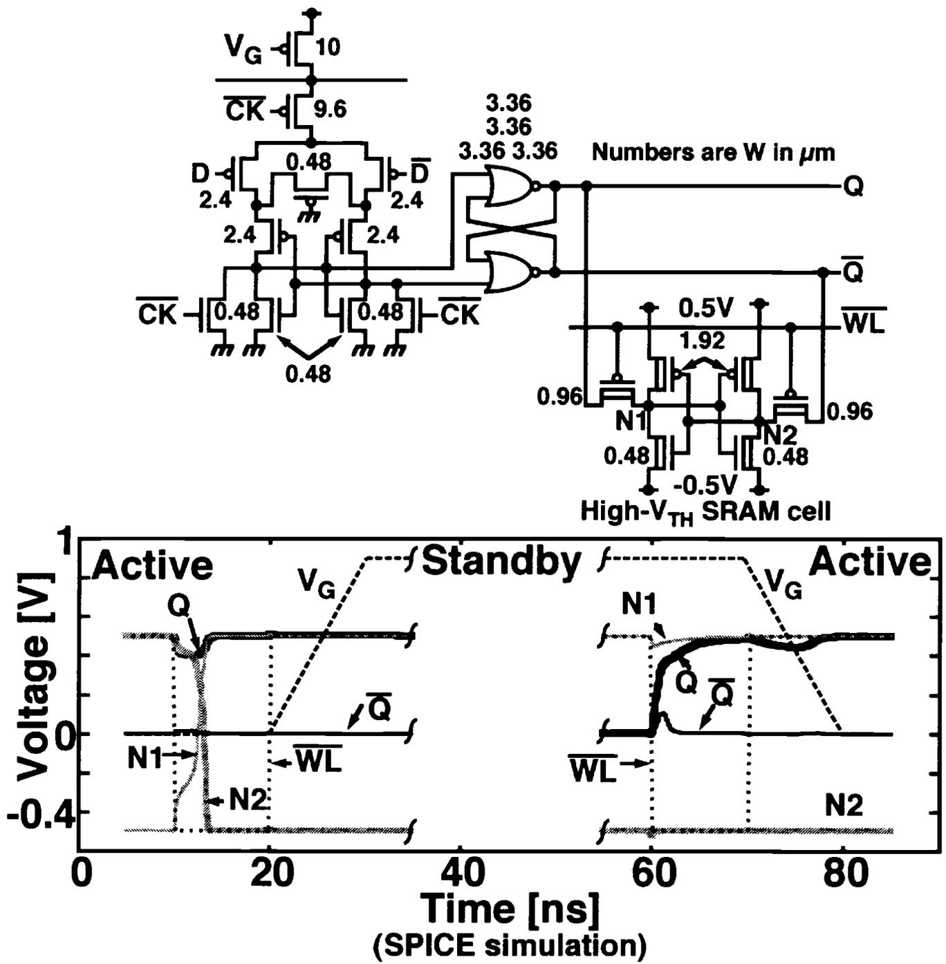
Figure 4: SCCMOS flip-flop and operating waveforms.
