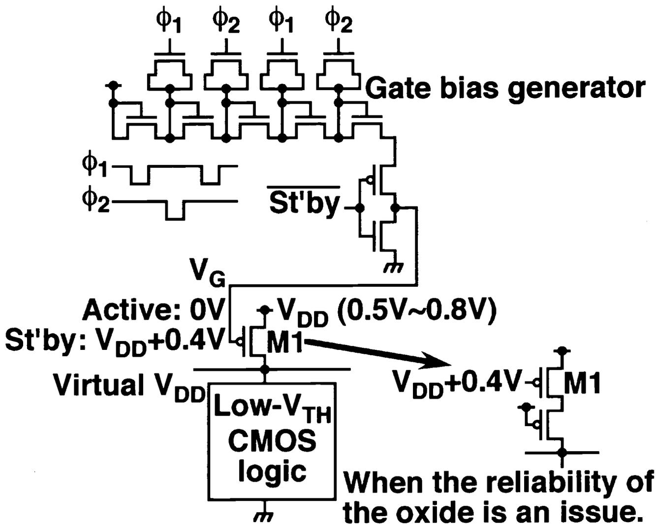
**Figure 1:** Super cut-off CMOS (SCCMOS) scheme.
