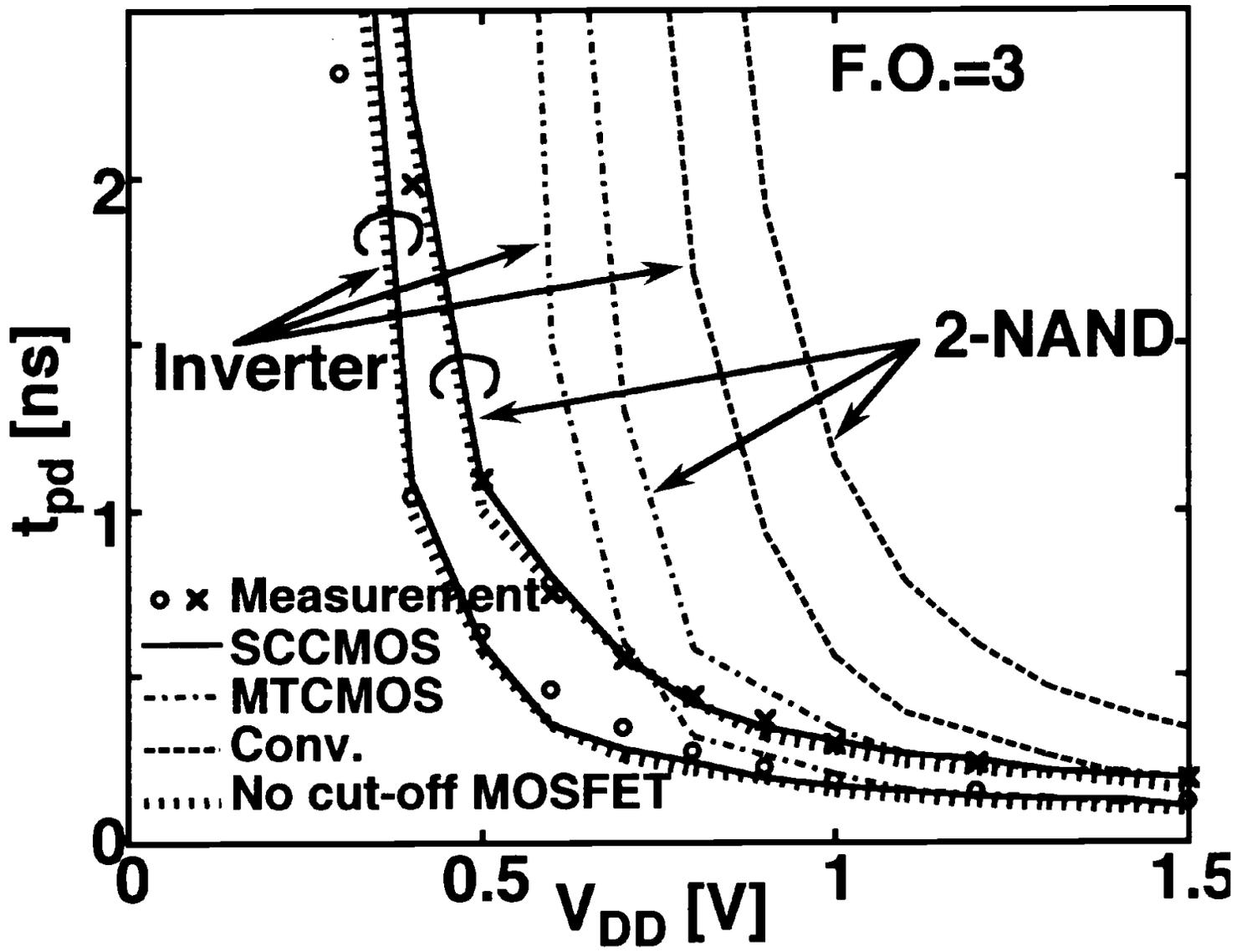
Figure 3: Speed of inverter and NAND with SCCMOS.
