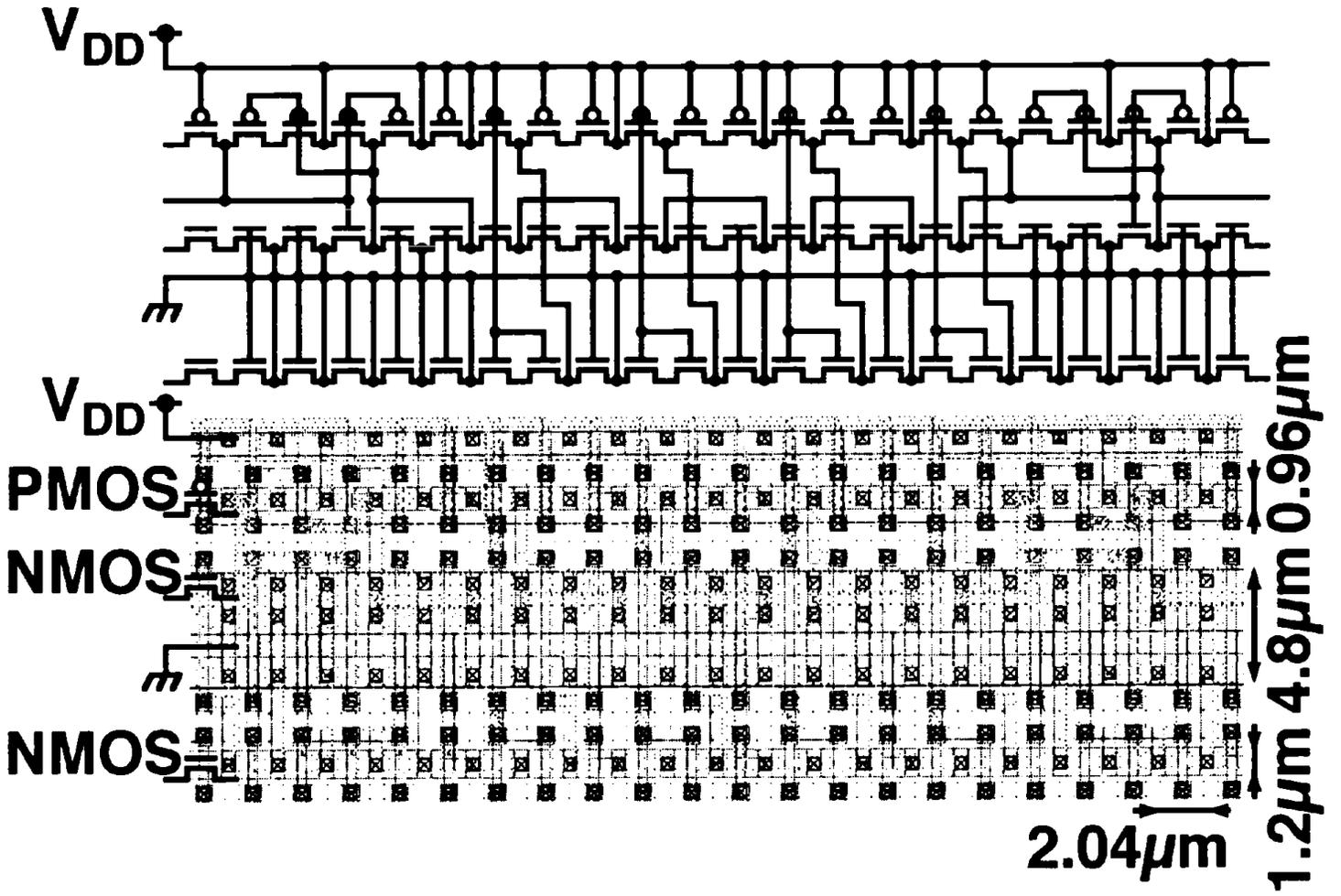
Figure 7: PTL oriented gate array.
