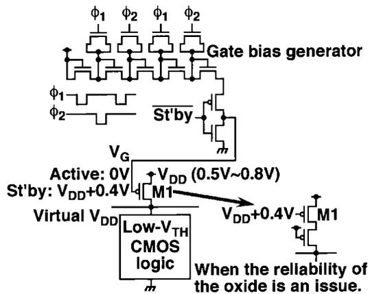
Figure 1: Super cut-off CMOS (SCCMOS) scheme.
