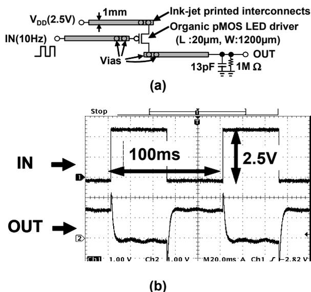
**Fig. 10. Measured waveform of organic transistor through printed interconnects. (a) Measurement set-up. (b) Input and output waveforms.**
