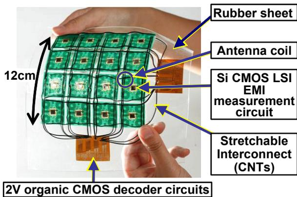
Fig. 3. Stretchable EMI measurement sheet.
