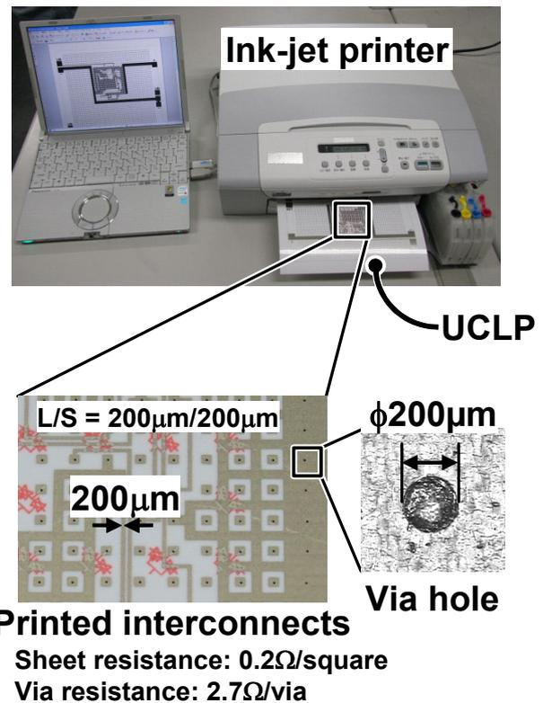
**Fig. 9. Photograph of the printing process of the interconnects on UCLP using ink-jet printer, printed interconnects, and a via hole.**
