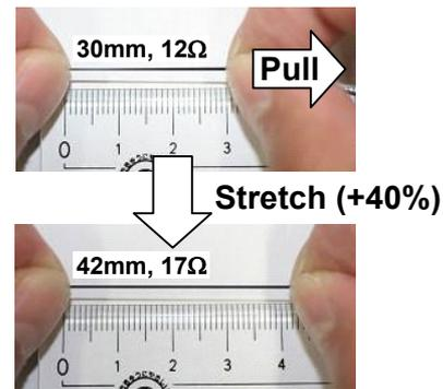
Fig. 5. Demonstration of stretchable interconnect.
