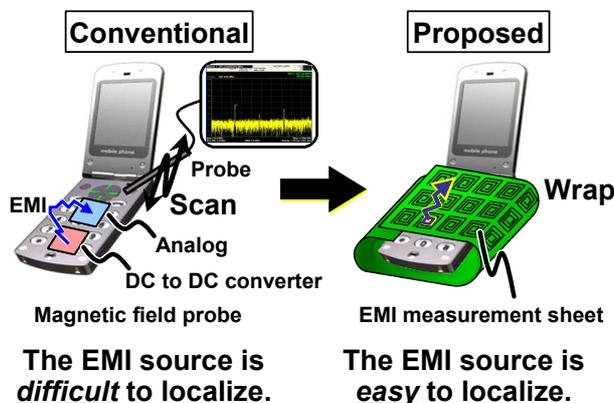
Fig. 2. Intrasystem EMC issue in a mobile phone.
