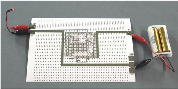
**Fig. 6. User Customizable Logic Paper (UCLP) for educational purpose. Learners can study and experience operation of integrated circuits by fabricating custom integrated circuits, using at-home ink-jet printers to print conducting interconnects on paper that contains prefabricated arrays of organic transistors.**
