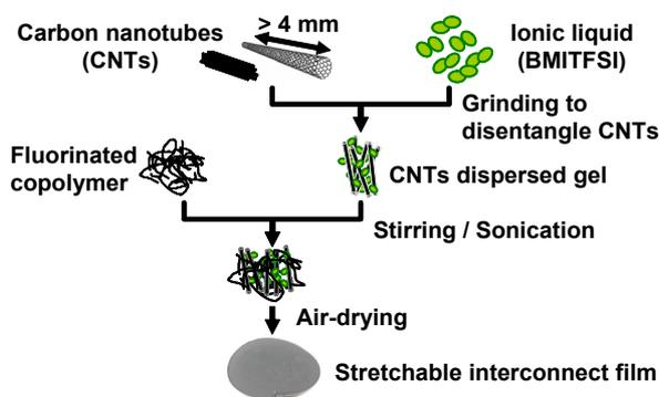
Fig. 4. Process flow of the stretchable interconnects.
