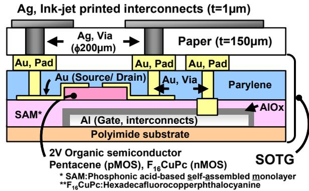
**Fig. 8. Cross section of UCLP.**
